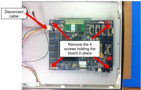
Grab the board from the top and carefully flip it. It is held on by 3 cables
